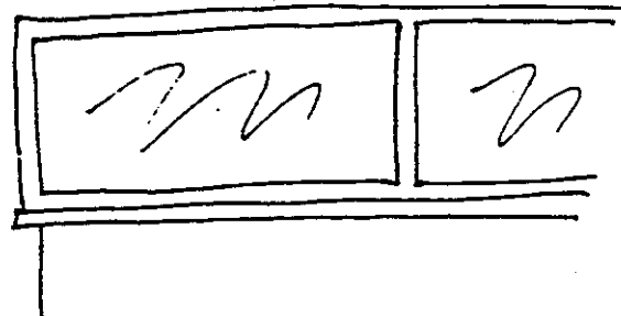
Box Case custom-sized with base one or more sections wood frame, glass top and sides
