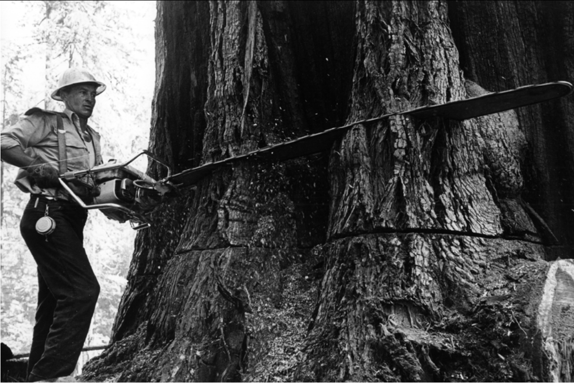
Figure 96. To cut the huge redwoods, extra-large chain saws were created. Compare to Figure 97. (Photo courtesy of Humboldt State University Humboldt Room collection.)
