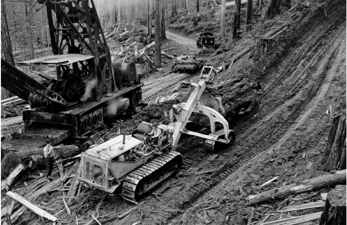
Figure 92. Tractors with "caterpillar" treads allowed dragging of the huge logs from the forest, but caused in much soil disturbance, resulting in erosion of soil into the streams. (Photo courtesy of Pacific Lumber Company.)
