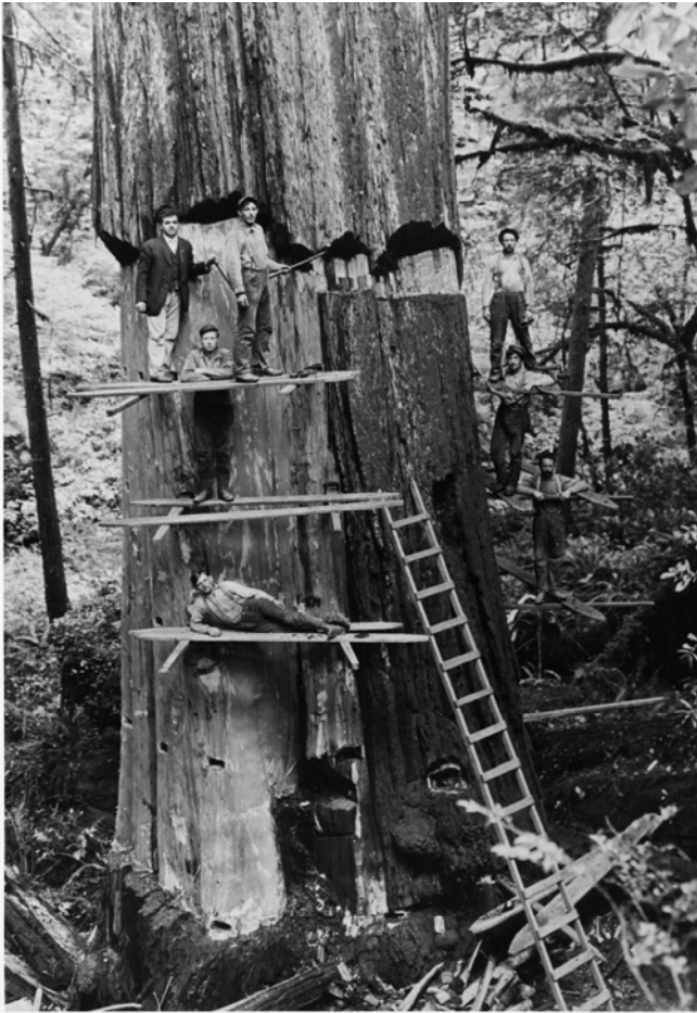
Figure 78. The wood at the base of a large redwood is often not as straight-grained as the rest of the tree, it may be harder, and it is often significantly greater in diameter than the trunk a few feet off the ground. Fallers cut notches in the thick bark and inserted spring boards to create a scaffolding or platform, sometimes ten or more feet off the ground. (Photo courtesy of the Humboldt State University Partain collection.)
