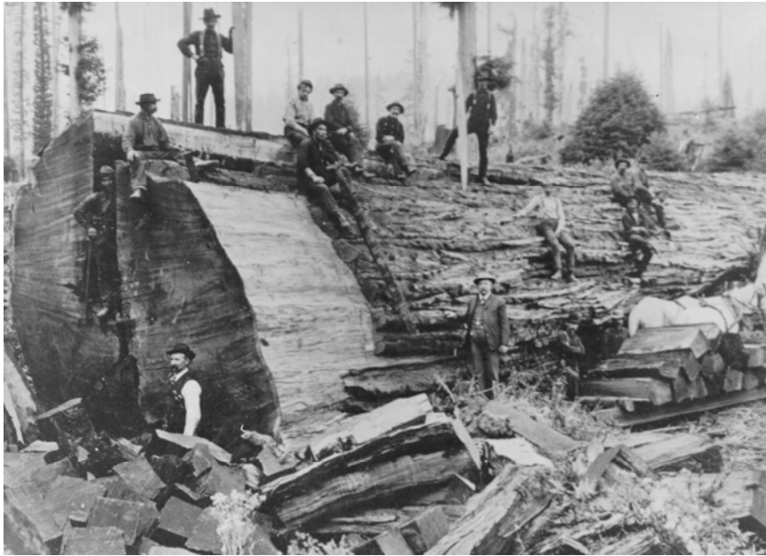
Figure 86. Huge trees were sometimes "bucked up" (cut into sections) with whip saws to make railroad ties, grape stakes, shingles, or other split goods. (Photo courtesy Pacific Lumber Company.)
