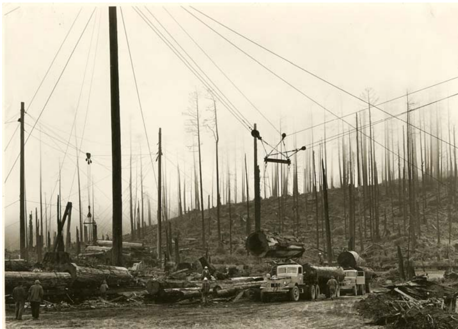
Figure 85. Sky-line cabling moves logs to landings with the whole log suspended on cables. Both high-lead and sky-line cabling systems require the removal of trees and brush along the route to prevent the logs and cables from getting tangled in the intervening trees. Compare this picture with Figure 97. (Photo courtesy Clarke Museum collection.)
