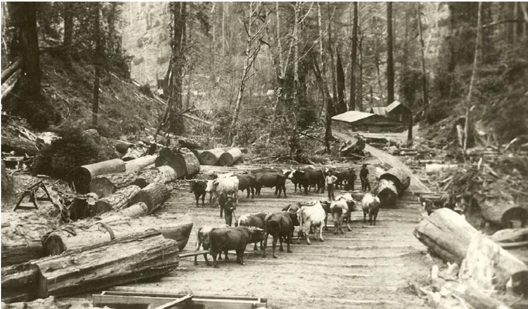
Figure 83. Oxen were often used to drag logs on the skid roads to the landings. Because travel was slow, loggers often lived in logging camps set deep in the woods. (Photo courtesy Clarke Museum.)
