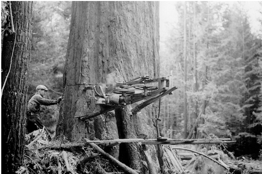
Figure 81. The gas powered drag saw proved cumbersome in the rugged north coast redwood range. (Photo circa 1940.) (Photo courtesy Pacific Lumber Company collection.)
