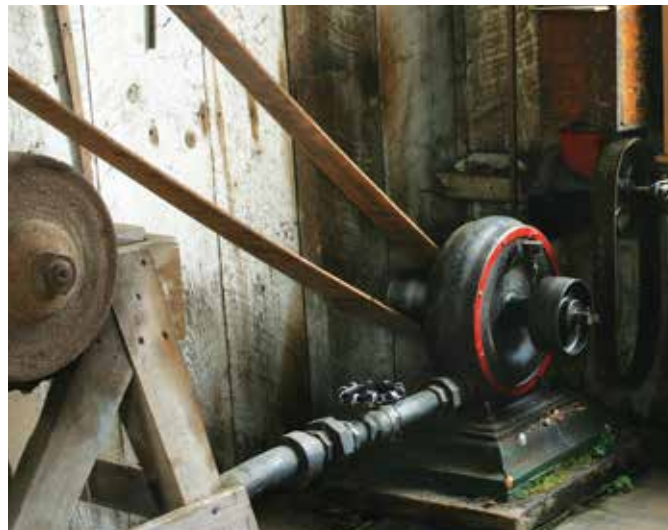
The Pelton water wheel drives the dairy and farm equipment.
