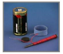
I found a lot of old telephone hookup wire to use for the coil of wire around the nails – so that is what is shown in the pictures. When you cut the light bulbs from the holiday light strings there is a lot of wire left over – that wire will work also. Don't use lamp cord wire – it's too thick.
