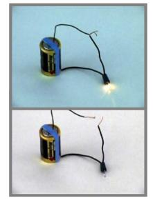
In the top picture on the right, the ends of the wire are twisted together so that we get a complete, "closed" circuit. The light bulb will light up. In
