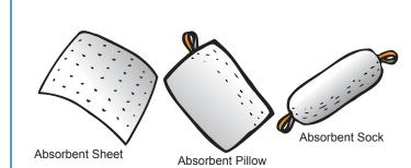
Absorbent Socks or Pillows in the Bilge: Socks and pillows are designed for use in deeper bilge compartments. Properly secure absorbents in the bilge. If you have an extremely oily bilge, consider using a bilge pumpout service and then a steam cleaning service that properly disposes of the wastewater.
