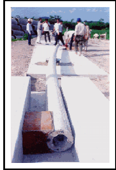
Flex Testing Spun Concrete Pile
