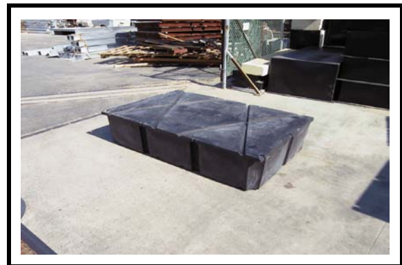
Roto-Cast Polyethylene Foam-Filled Pontoon
