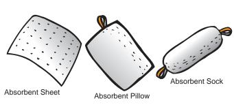
Absorbent Socks or Pillows in the Bilge: Socks and pillows are designed for use in deeper bilge compartments. Properly secure absorbents in the bilge. If you have an extremely oily bilge, consider using a bilge pumpout service and then a steam cleaning service that properly disposes of the wastewater.
