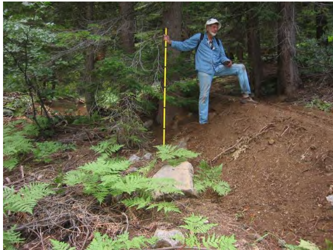
Depth and width of Freeman Creek Trail cut (pole segments are 1 foot each)
