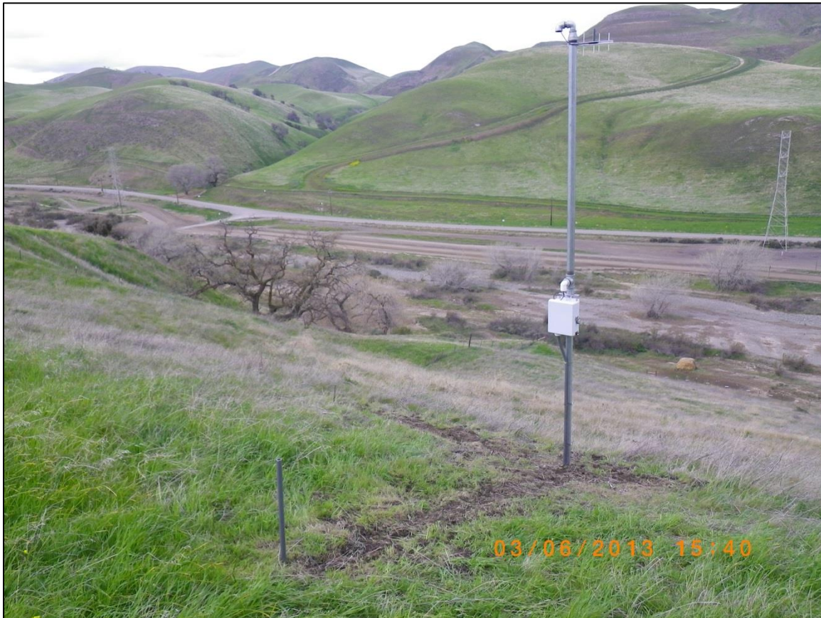
Figure 10. Soil Moisture Meter at Site 5. The meters were installed in March 2013 at five locations.
