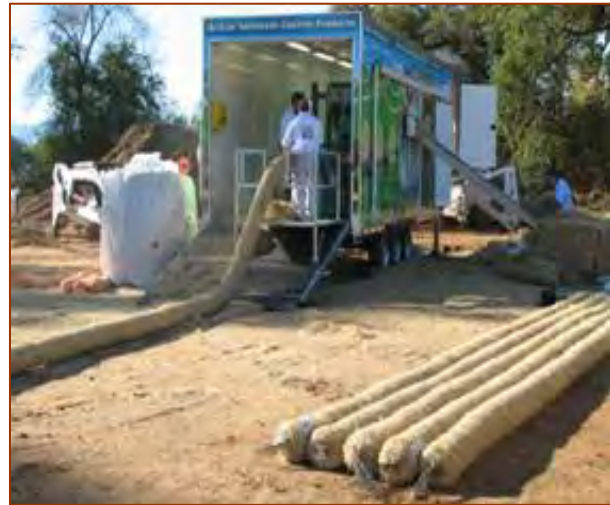
This portable trailer manufactures fiber rolls on-site and can produce any length of roll.
