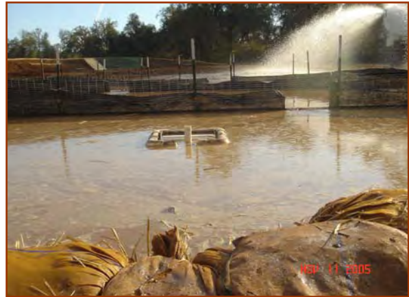
The skimmer drains the basin from the top, where the stormwater is cleaner (BMP testing at the Shasta College Erosion Control Training Facility, 2005).
