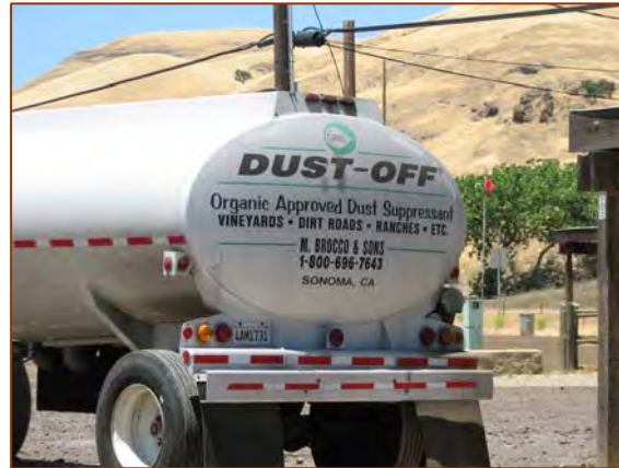
Organic dust suppressants can be used to control dust and stabilize soil. (Carnegie SVRA)
