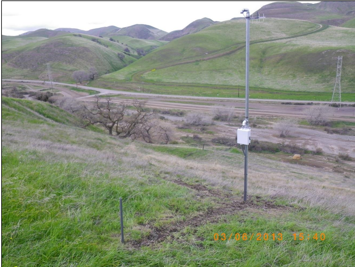
Figure 12. Soil Moisture Meter at Site 5. The meters were installed in March 2013 at five locations.
