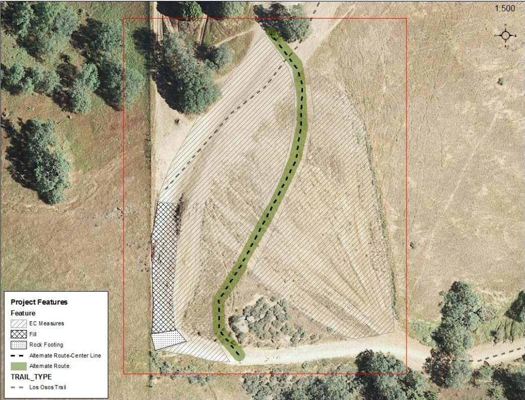
Map 6. Through-cut. Improvements included re-aligning the emergency access road, rehabilitating the areas adjacent to the road, and fencing to exclude off-highway vehicle access in the future.
