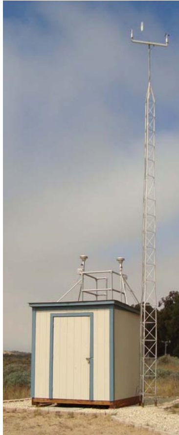
Figure 2-10 Example FEM Monitor with Shelter and 10-Meter Tall Lattice Tower.
