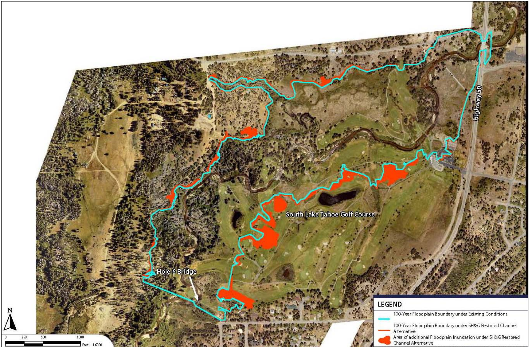
Boundaries of the 100-Year Floodplain under the SH&G Restored-Channel Alternative versus Existing Conditions
