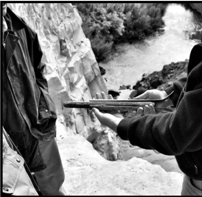
Plug and Feather Device Still in Use Today to Split Sandstone
