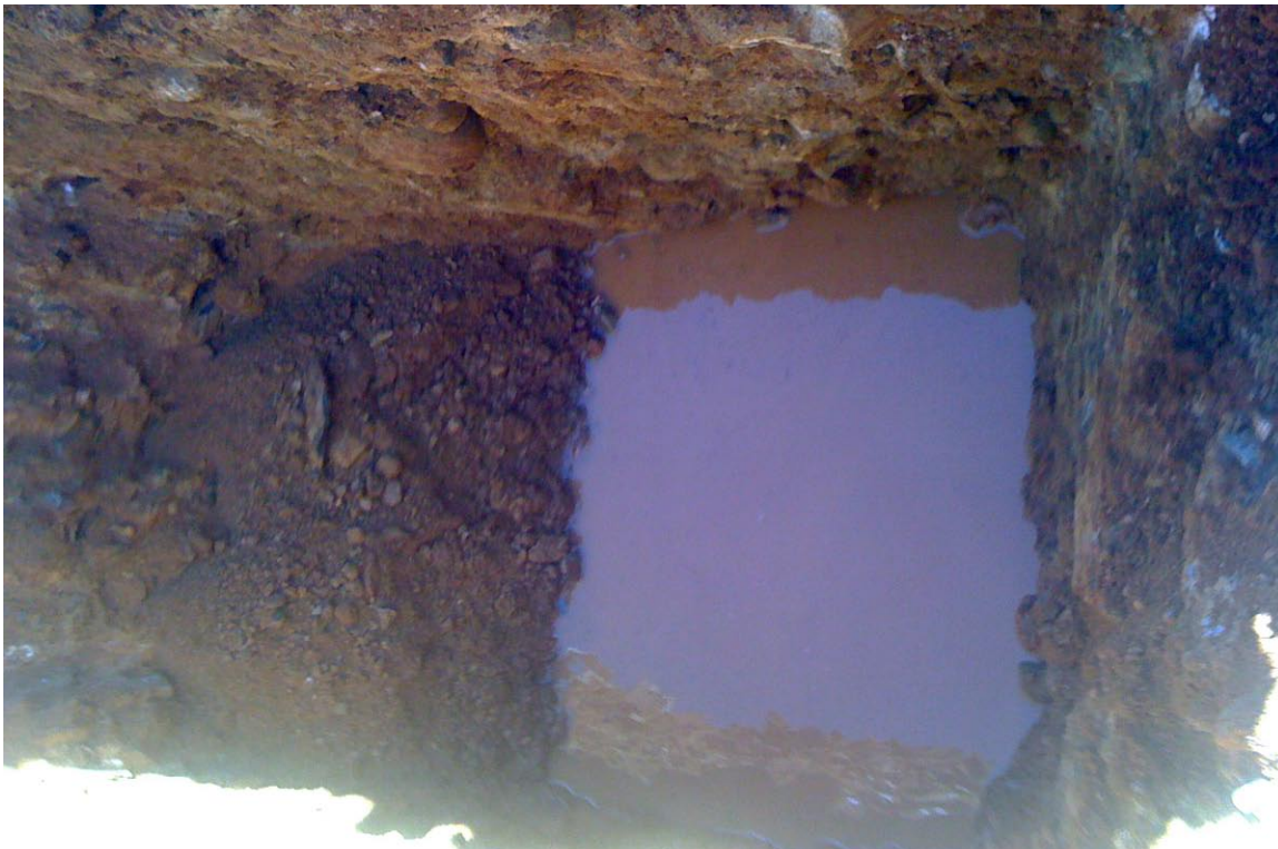
Photo No. 4 Percolation Test in Pit
