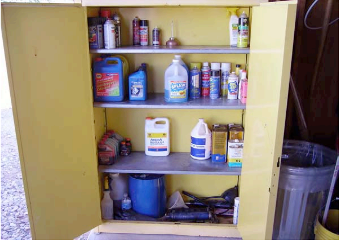
Photograph 9. View of flammable locker storage for oil, paint, cleaners; blue container at lower left used for small quantities of waste oil picked up by rangers.
