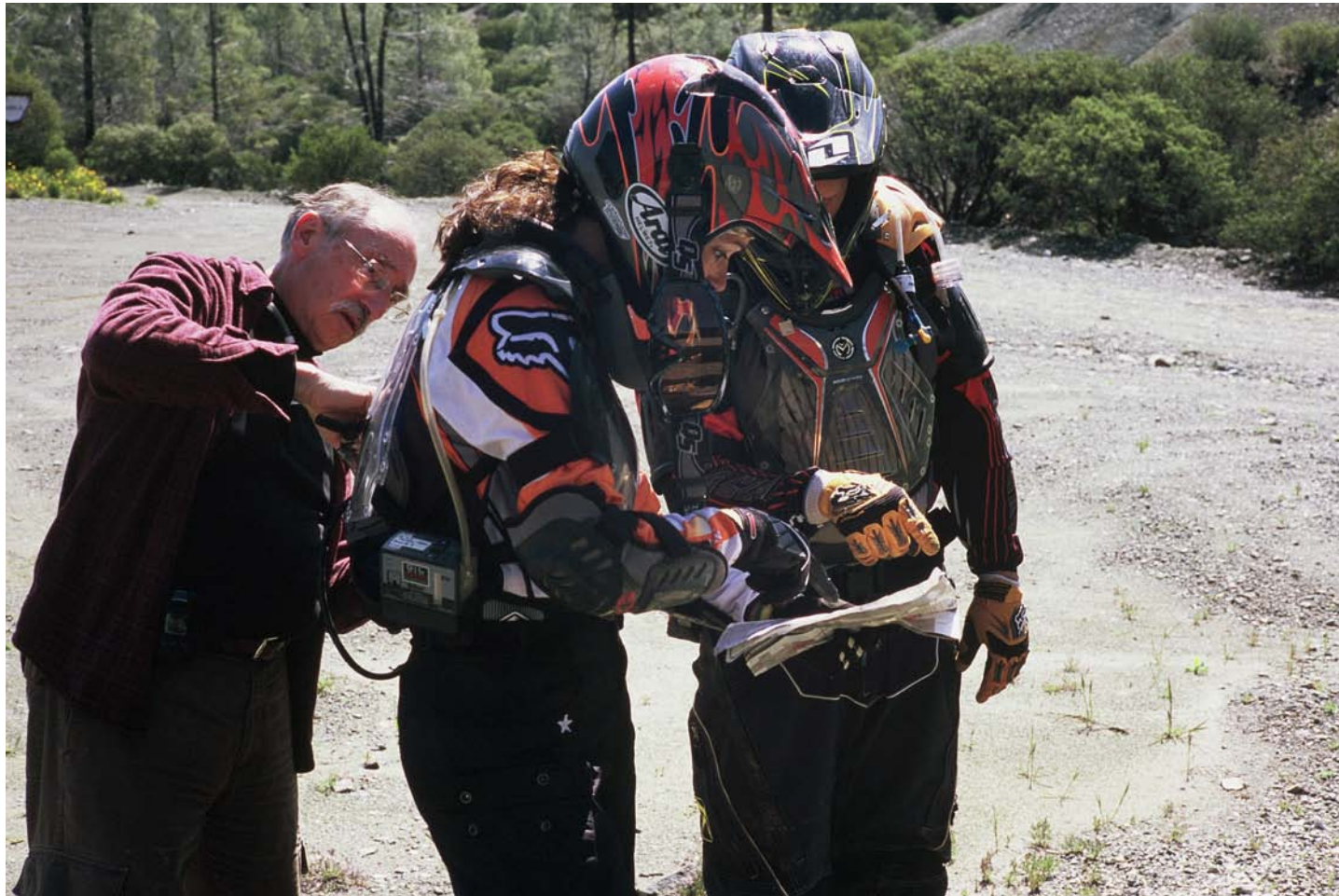
Figure 7. The industrial hygienist is placing air-sampling pumps (with air filter cassettes) on the two riders. The personal air samples were collected about chest high as the two rode the trails. It is assumed, collecting airborne particle here is equivalent to the air they are breathing, but the motorcycle helmets the riders wear may mean this assumption is incorrect.
