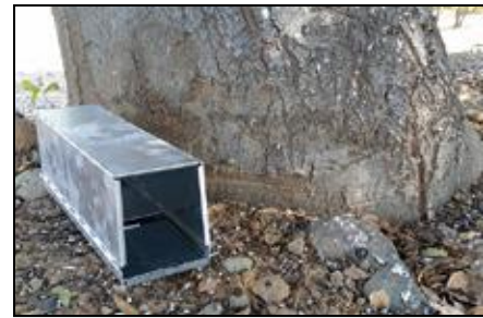
Sherman trap designed for the live capture of small mammals
