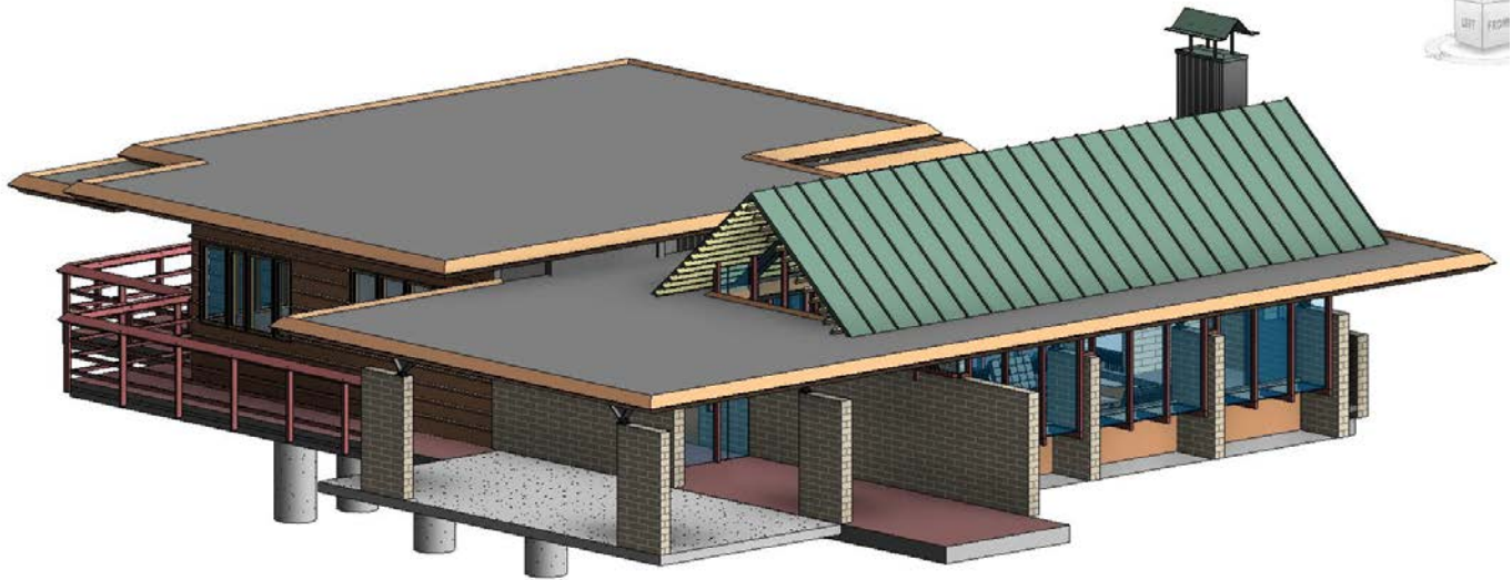
Illustration 1. Front view of house with covered carport in the foreground, and standing seam copper roof over living room. Revit model by Thomas Rex Hardy, AIA.
