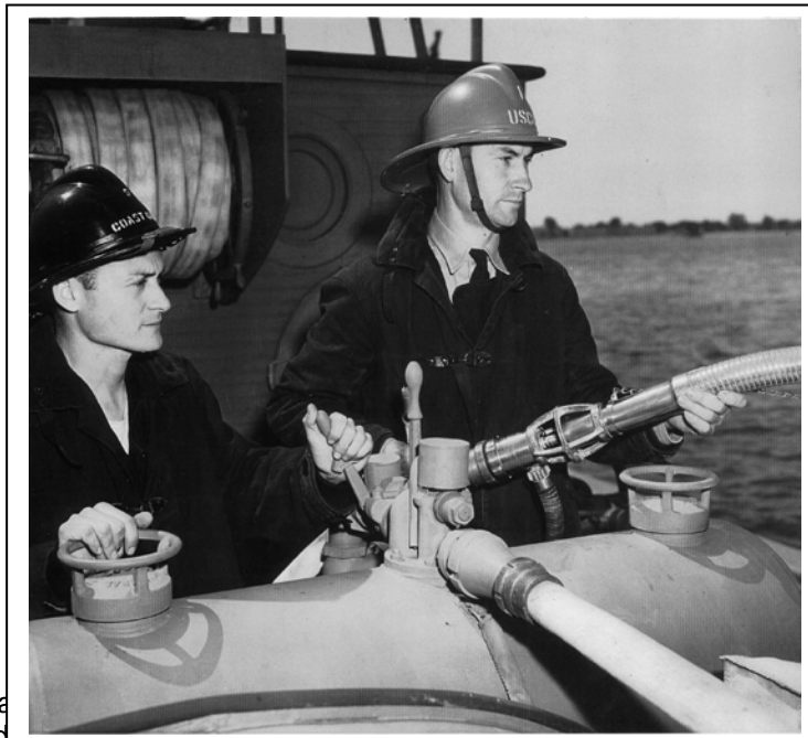
(Image 27: When Chief Ely invented the Ely Adapter, designed to function as a stream nozzle. It would only be the first of many creations Ely would provide the fire service.)
