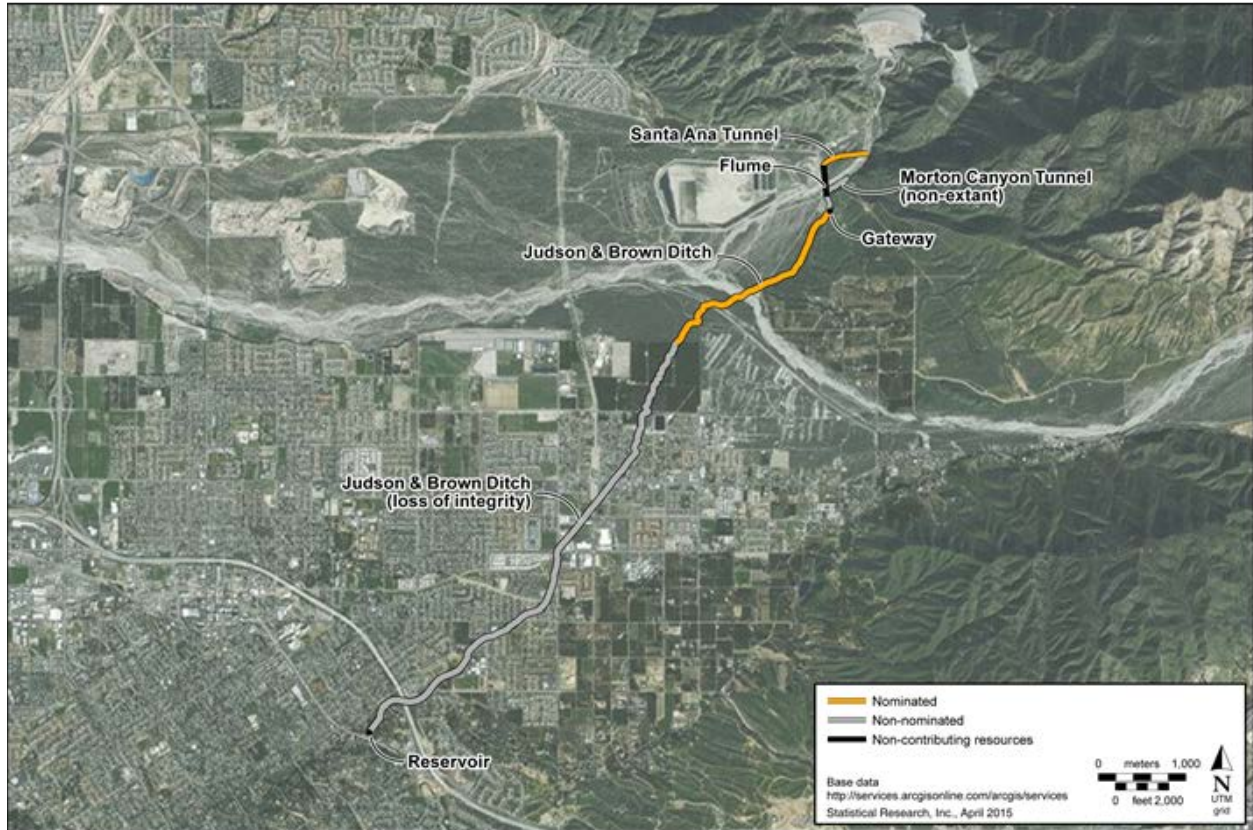
Figure 2. Map of Right-of-Way of Judson and Brown Ditch, showing the water's right-of-way including tunnels, flumes, and the canal to the reservoir.
