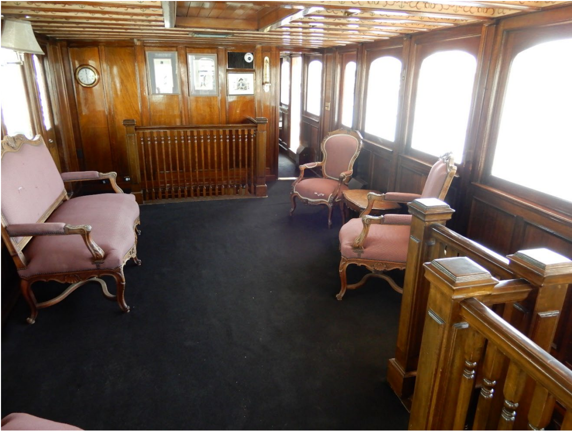
Figure 18. Parlor at aft main deck, showing fore and starboard wall, with non-original stair, stenciled ceiling beams, and former location of stained-glass skylight visible (ARG, 2022)
