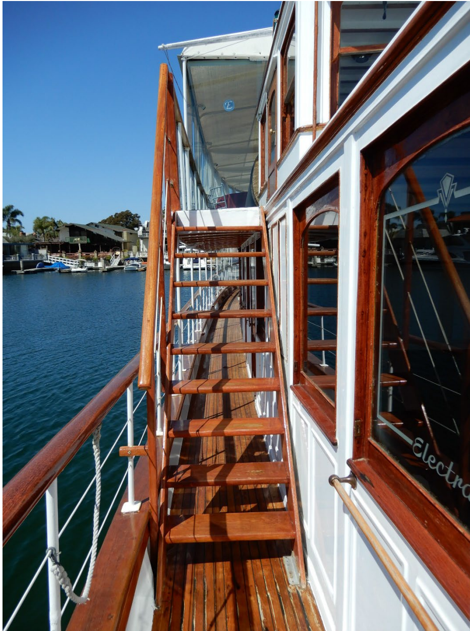
Figure 10. Starboard side promenade deck at main deck, showing non-original stair to pilot house (ARG, 2022)
