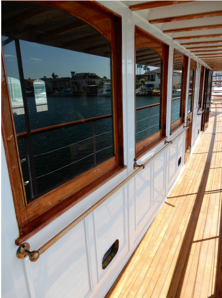
Figure 11. Starboard side promenade deck at main deck, showing mahogany cabin finish details (ARG, 2022)
