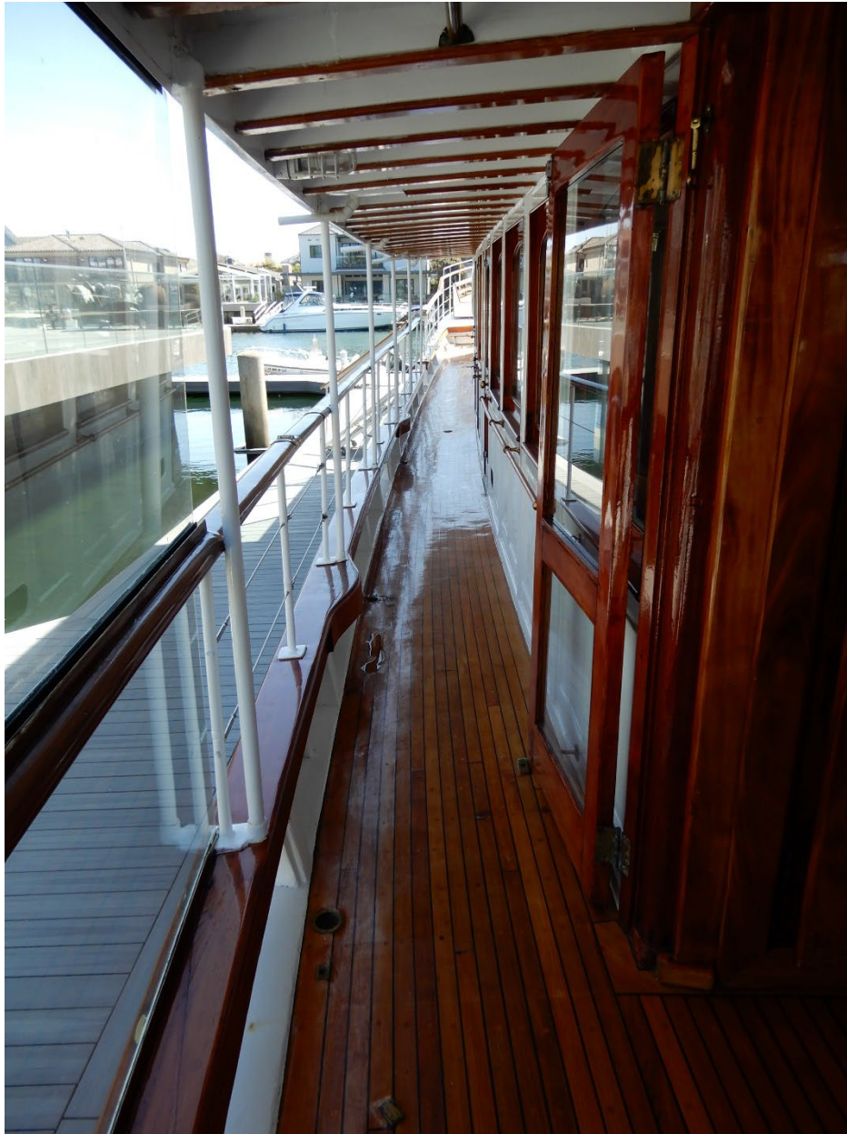
Figure 09. Portside promenade deck at main deck, showing teak decking (ARG, 2022)
