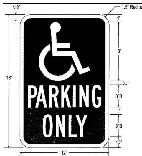
Figure 26-4 Accessible Parking Sign
